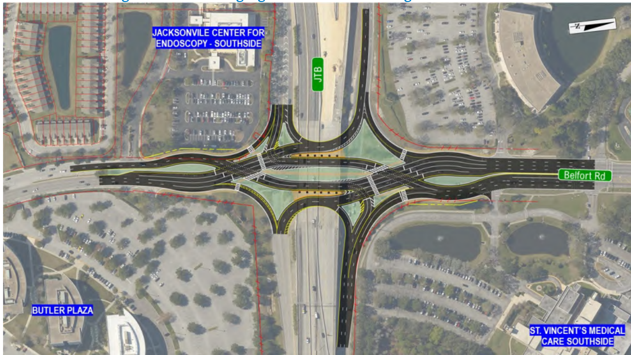
Figure 3.2.1: Diverging Diamond Interchange at Belfort Road
